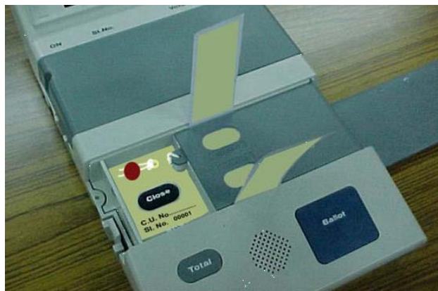
ECIL Machine Sealing the inner door with Special Tag
